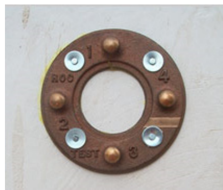
樓宇監察裝置 Building Monitoring Device
