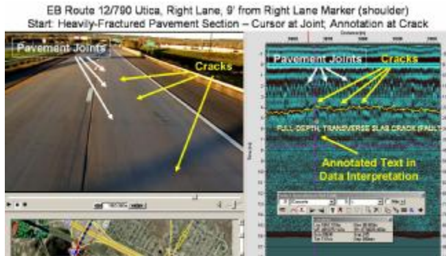
Fig. 8. Linking Surface Features to Subsurface Features with Road Doctor
