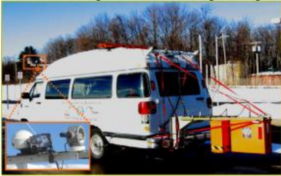
Fig. 4. Vehicle Equipped for Performing High-Speed GPR Surveys. Equipment Includes Air-Horn GPR Antennas (Bottom Right), GPS, Video, and Positioning Laser (Bottom Left)
