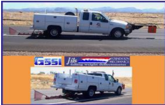
Fig. 3. JILS System with FWD, GPR and GPS
