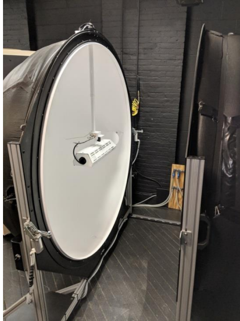
Figure 3. Integrating sphere used to measure absolute light output at 25° C.
