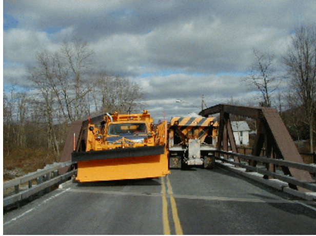
Figure 13. Trucks A and B in position - Load Case 1.
