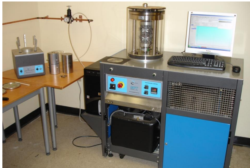
Figure 2 – Photo of the Asphalt Mixture Performance Tester (AMPT)
