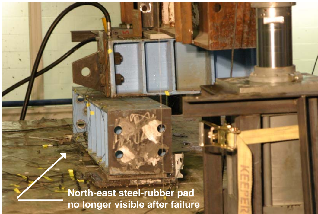
Fig. 5.5 Photograph of spreader frame and failure at north-east load point
