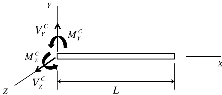
Fig. 5.16 Forces acting at mast arm connection for Group II and III load combinations.
